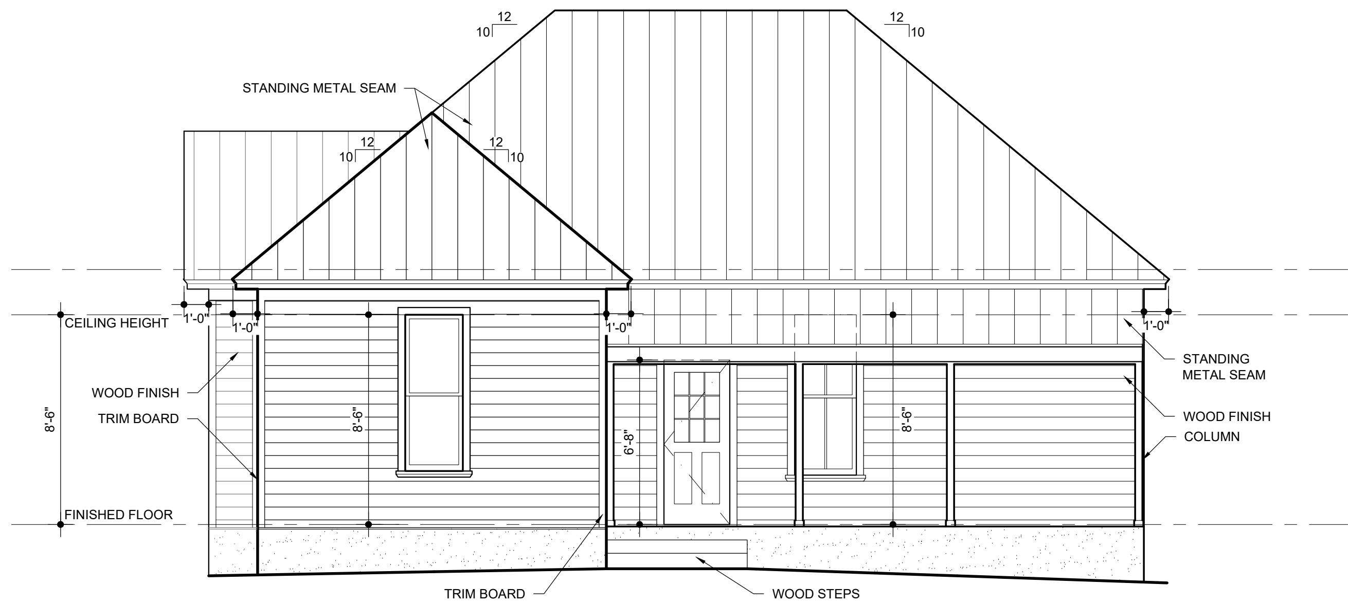
3 BACK ELEVATION A-21 1/4"=1'-0"
